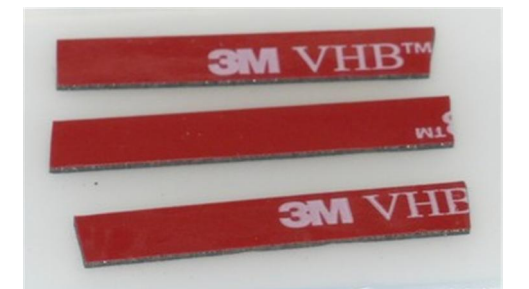
3M VHB tape to secure wires
